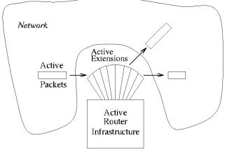
Active router infrastructure is a secure environment that supports the execution of the upper layers - switchlets, and PLAN packets. Basic services such as routing, address resolution, forwarding, and even PLAN interpretation are implemented as switchlets. The entire Switchware architecture is based on Caml, both as a development language for the extensions, and as a base for PLAN. Its main advantage is strong static typing, and compilation to bytecode.
