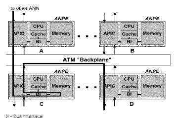
A capsule received on port A is forwarded to C, and then to D, and its execution will take place in the least loaded ANPE. APICs support zero copying semantics, therefore no copying is performed from the network to the execution environment.
