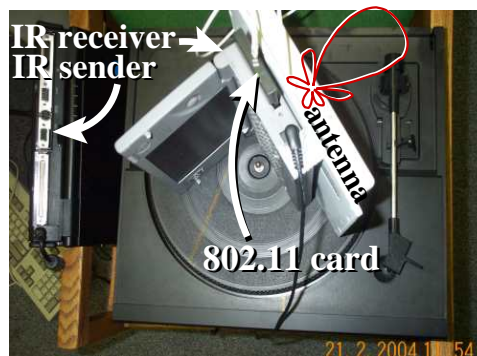
Figure 2: Experimental base station with revolving antenna
