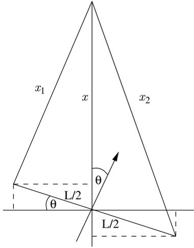
Fig. 2. Basic principle of Cricket Compass (adapted from [6]).
