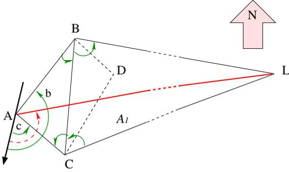
Fig. 4. Node  $A$  estimates its bearing/radial/range to  $L$  by corroborating  $B$ 's and  $C$ 's estimates.
