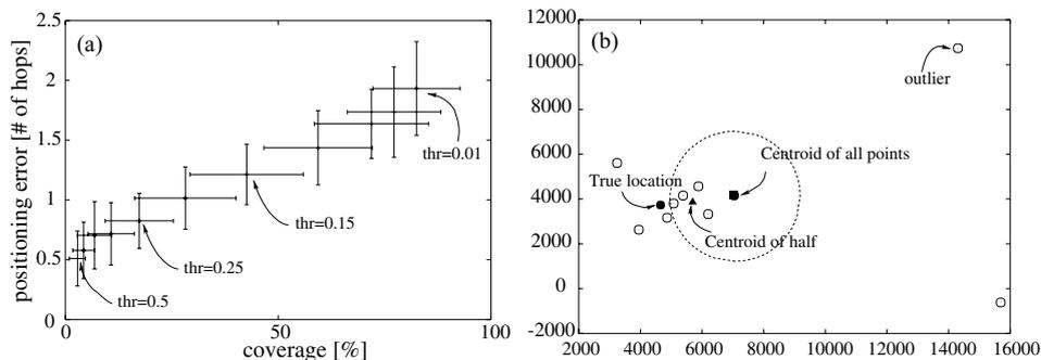
Fig. 9. (a) Angle threshold: tradeoff error-coverage. (b) Removing outliers from centroid computation.
