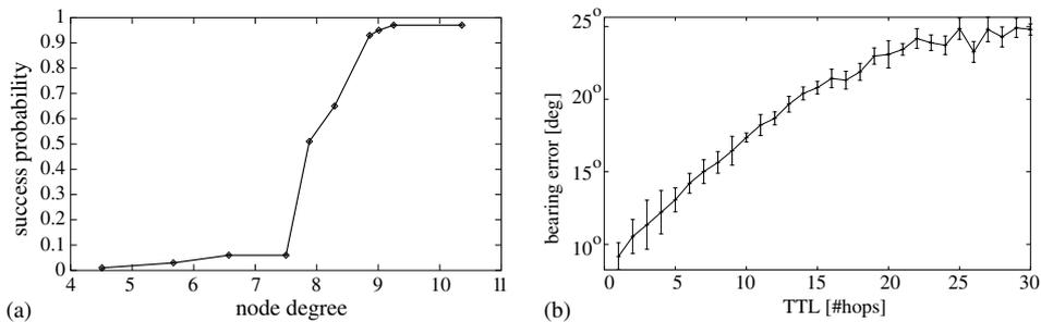
Fig. 8. (a) Probability for a node to satisfy conditions necessary for forwarding. (b) Error is compounded with propagation.
