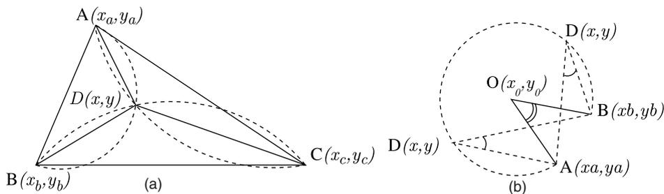
Fig. 3. Positioning using angles or ranges to landmarks. (a) Triangulation and trilateration. (b) Geometric locus of a point seeing two known landmarks at a given angle, is a circle.  $\widehat{AOB} = 2\widehat{ADB}$ .
