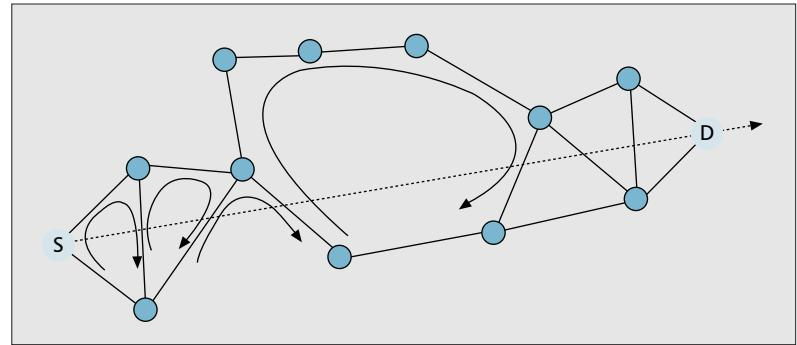
■ Figure 4. The FACE algorithm routes around obstacles using the lefthand rule.
