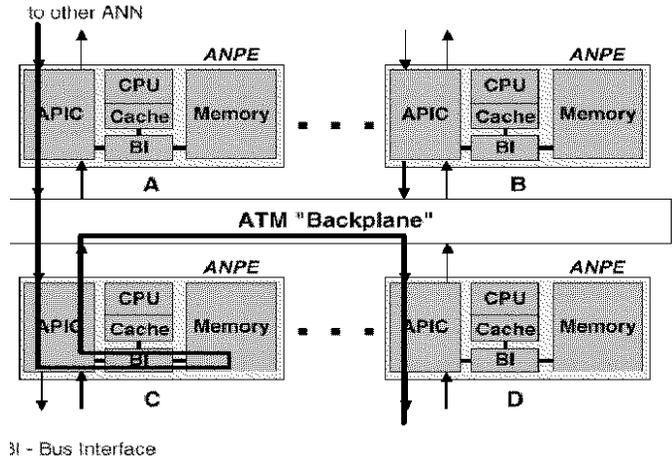
A capsule received on port A is forwarded to C, and then to D, and its execution will take place in the least loaded ANPE. APICs support zero copying semantics, therefore no copying is performed from the network to the execution environment.
