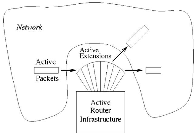
Active router infrastructure is a secure environment that supports the execution of the upper layers - switchlets, and PLAN packets. Basic services such as routing, address resolution, forwarding, and even PLAN interpretation are implemented as switchlets. The entire
