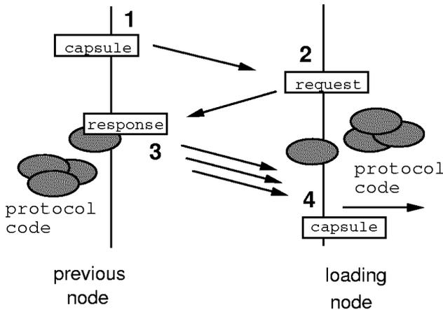
The on-demand scheme increases the startup latency of the protocol, other possibilities being to preload the code in advance or to carry the code in each capsule. On the other hand, it has the advantage of being adaptive to network failures and appropriate for short lived
