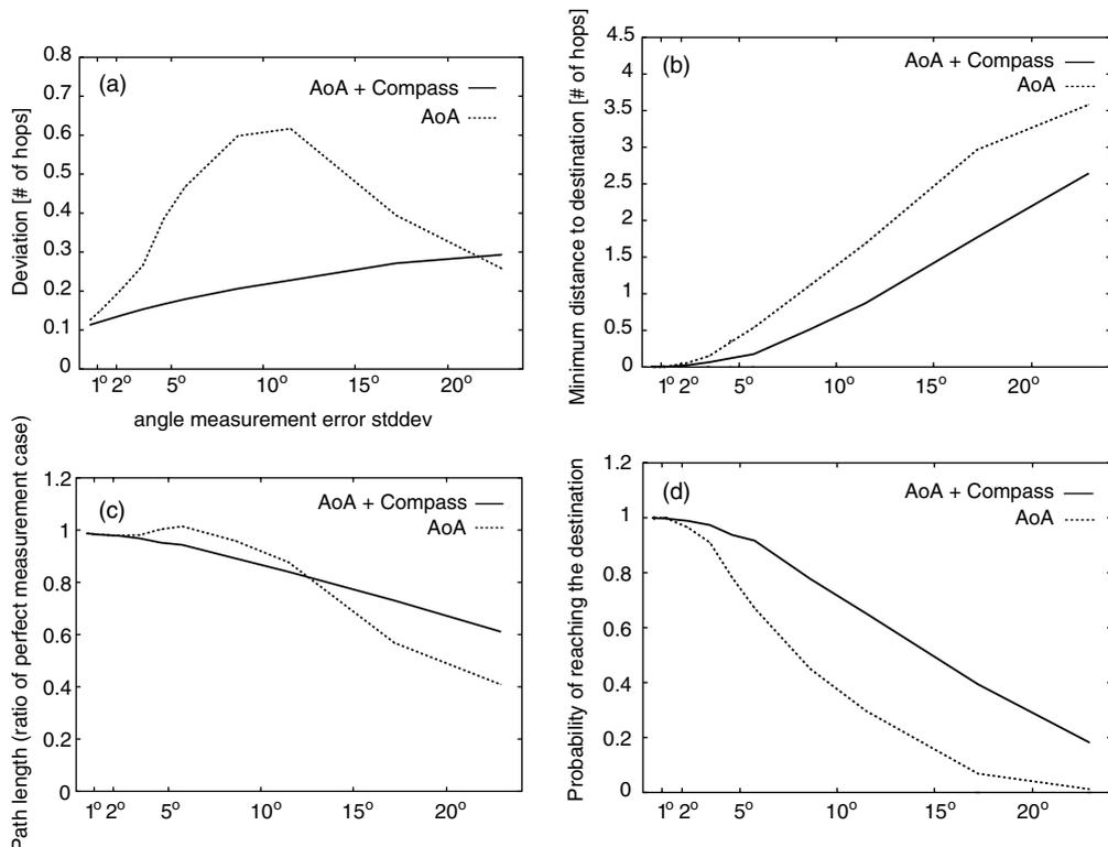
Fig. 5. AoA, AoA + compass. (a) Deviation from 'perfect' trajectory, (b) minimum distance to destination, (c) path length—relative to 'perfect' trajectory, (d) probability of reaching the destination.
