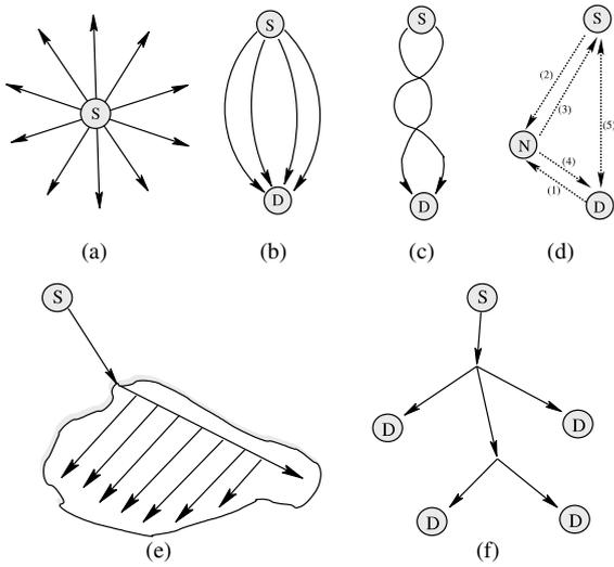
Fig. 1. Trajectory based flooding, routing and discovery.
