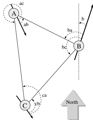
Fig. 2. Nodes capabilities: measuring angles, ranges, orientation.
