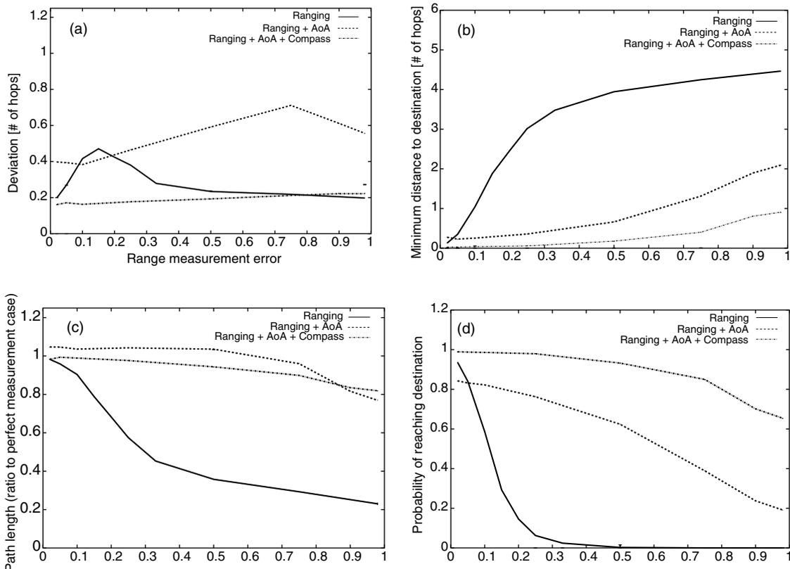
Fig. 4. Range, range + AoA, range + AoA + compass. (a) Deviation from ‘perfect’ trajectory, (b) minimum distance to destination, (c) path length—relative to ‘perfect’ trajectory, (d) probability of reaching the destination.
