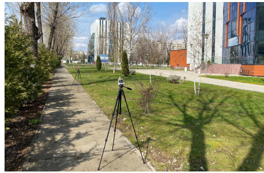
Fig. 2. Location at which the range of the devices was measured. The devices were placed at distances between 5 and 220 m along the pathwalk.
