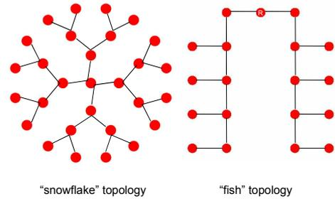
Fig. 4. Topologies used for evaluation: "snowflake" topology can be used as an access network for a circular area; "fish" network for a rectangular area.
