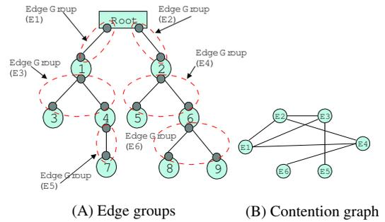
Fig. 2. (A) Creation of contention graph with the following interface model: Edge groups interfere if they have a common node; nodes 1 and 2 interfere (less than carrier sense distance). (B) Edge groups become nodes in the contention graph
