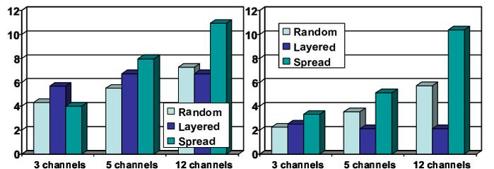
Fig. 6. Performance [Mbps] for "fish" topology. each card at the root can handle 6Mbps (1.5Mbps per leaf). left: unidirectional, optimal=10.95Mbps right:bidirectional, optimal=10.38Mbps
