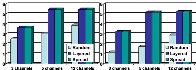
Fig. 7. Performance [Mbps] for string topology. Left: unidirectional Right:bidirectional. 4 channels are necessary for all hops to operate at maximum capacity.
