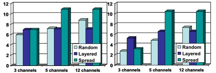
Fig. 5. Performance [Mbps] for "snowflake" topology: each card at the root can handle 6Mbps (750Kbps per leaf). Optimal throughput=10.94Mbps. left: unidirectional right:bidirectional
