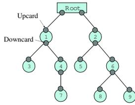
Fig. 1. A wireless mesh network with tree topology
