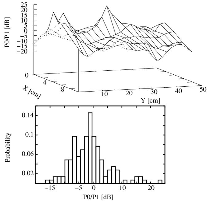
Fig. 9. Upper: gain difference at the receiver antenna between the two sending antennas. The receiver antenna takes different positions one grid spanning a  $500\text{cm}^2$  area. Lower: Power difference distribution histogram. 11% of the points exhibit more than  $10\text{dB}$  absolute difference in the power received from the two sender antennas.
