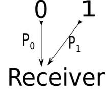
Fig. 7. Each of the sender antennas emits a different tone - and their power is recorded at the destination antenna.
