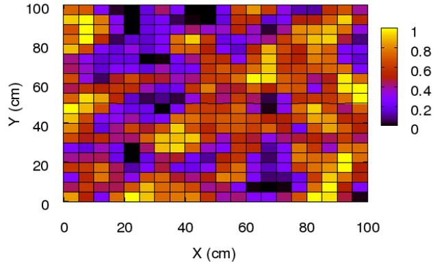
Fig. 2. Packet delivery ratio is measured from a robot mounted access point that changes positions across a  $1m^2$  grid. The access point and the receiver are fixed for each measurement.
