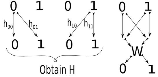
Fig. 6. The receiver uses both antennas for all the runs. The first run estimates  $h_{00}$  and  $h_{01}$  by only exciting antenna 0 at the sender. The second run estimates  $h_{10}$  and  $h_{11}$ . The third run uses the estimated channel to demodulate the distinct streams sent from each antenna.
