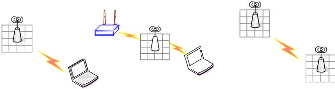
Fig. 1. Applications for mobile antenna/mobile element technique: at access point, for mostly static clients; at relay points to optimize both links; at long term point to point outdoor links.
