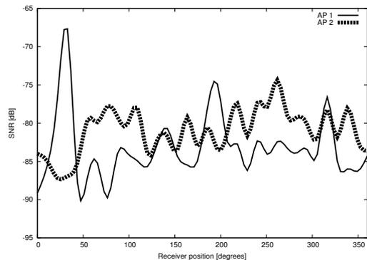
Fig. 3. A client rotating around its own axis can find a signal up to 20dB stronger. Both access points and the client are fixed for each measurement.
