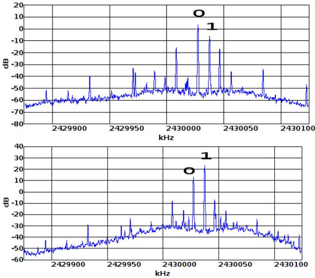
Fig. 8. FFT of two tones as seen at antenna 0 (top) and antenna 1(bottom). The tones are sent from the antenna 0 and 1 respectively at the sender. This is an uncorrelated, high capacity MIMO channel.
