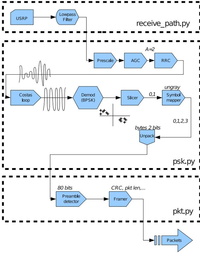
Fig. 5. BPSK receiver block diagram for each antenna. Channel estimation matrix linking the two streams gets plugged in between the demodulator and the hard decision slicer.
