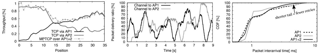
(a) Throughput of a client moving between  $AP_1$  and  $AP_2$ : the MAC favors the sender with the better channel. Max throughput is 22Mbps. (b) A fixed node has channels with a raw PDR $\approx$ 50% to each AP. The two channels are weakly correlated. (c) Packet inter-arrival rate exhibits a longer tail when a single AP is used. When both APs are sending, the tail is much shorter.
